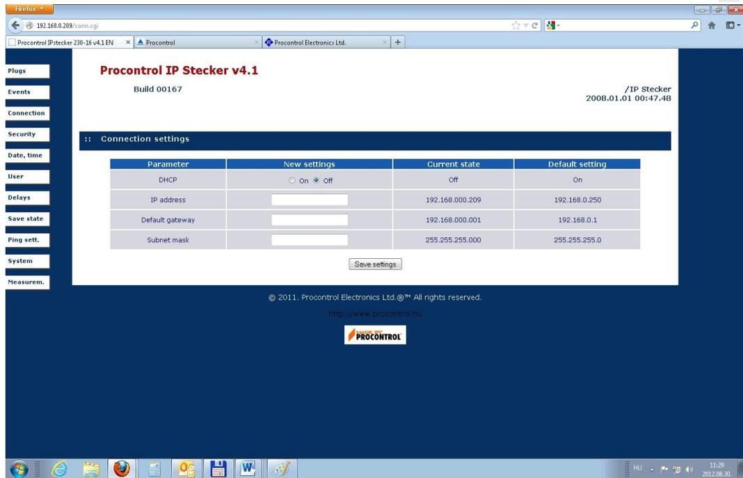
The screenshot shows the web interface of the Procontrol IP Stecker v4.1. The page title is "Procontrol IP Stecker v4.1" with "Build 00167" and "/IP Stecker 2008.01.01 00:47:48" displayed. The left sidebar contains navigation options: Plugs, Events, Connection, Security, Date, time, User, Delays, Save state, Ping sett., System, and Measuram. The main content area is titled "Connection settings" and contains a table with the following data:
