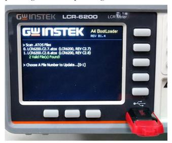
9. After you have pressed a number key that corresponds to the desired firmware file, the meter will show information about the chosen firmware file on the display. You can then confirm that the selected file is the correct file. If the selected file is correct, press the Enter key to confirm the selection and start flashing the firmware. Do not turn the power off when the firmware is being flashed. Pressing the ESC key will cancel the
